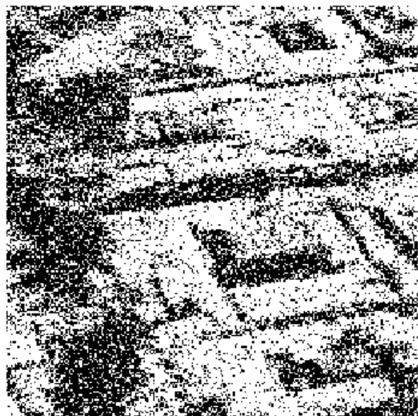
Figure 2 – Noisy, 8-bit simulated infrared image (frame rate = 320 Hz) and 1-bit thresholded image.
